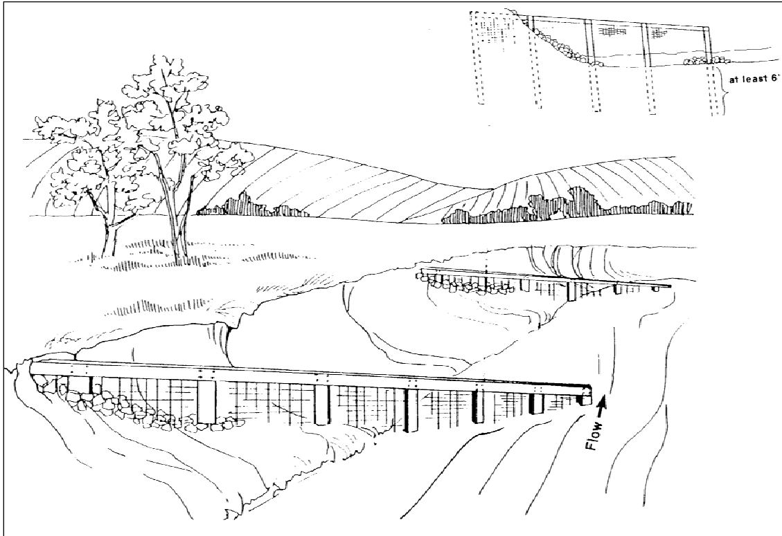
Figure 3.22. Jetties (Source: Department of Civil, Construction, and Environmental Engineering, Iowa State University)
